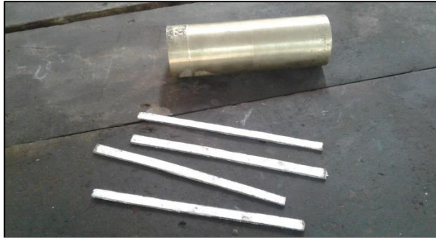
2. Figure 1: Composite (Al+SiC) rectangular fins with brass pipe
