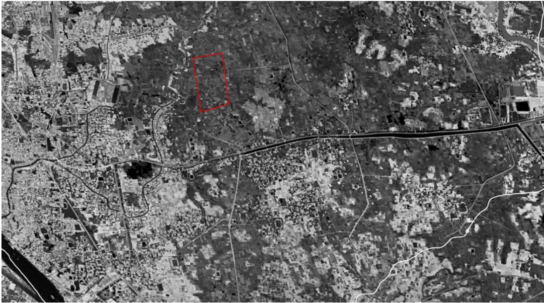
Fig 6: The present day layout of the Matuail landfill site overlaid on the CORONA satellite image of 1972, showing the position of the site within the wetland area of eastern Dhaka.
