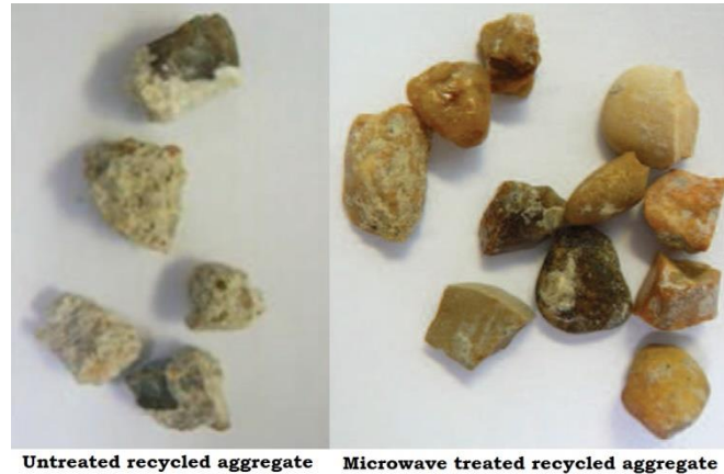
Figure 3. Untreated vs Microwave treated recycled aggregate. Bru et al (2014)
